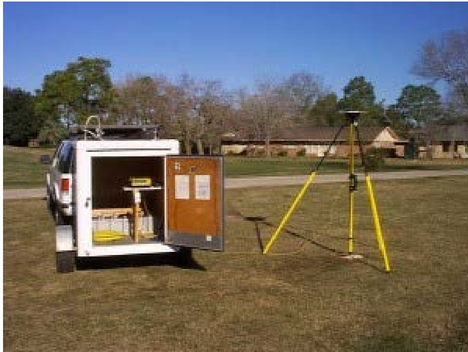
Figure 3-4 Picture of a Port-A-Measure (PAM) GPS antenna (modified from Zilkoski and others, 2003, obtained from https://hgsubsidence.org/frequently-asked-questions/measurement-FAQs )
